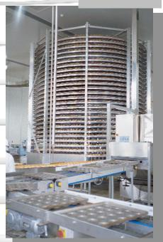
**Try this simple test:** With the Spiral "Off and Locked Out" try pulling the Spiral Belt away from the Cage by hand. It should pull away easily without much effort. If the Spiral Belt cannot be moved, if it feels extremely tight, or if it takes a lot of force to move, then the belt is most likely under High Tension.
